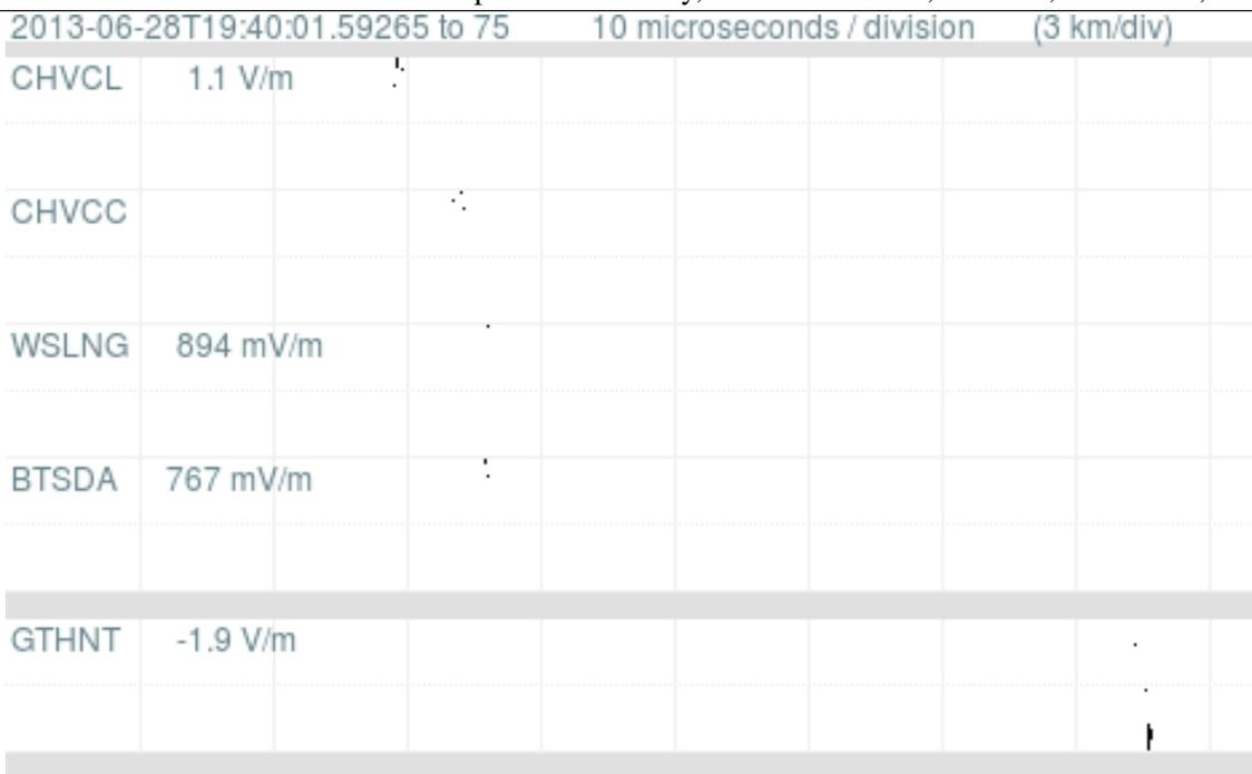
Figure 23: Electric field for seventh pulse. This is barely visible over the noise, and is only seen at 5 sites, so the location errors will probably be large.
