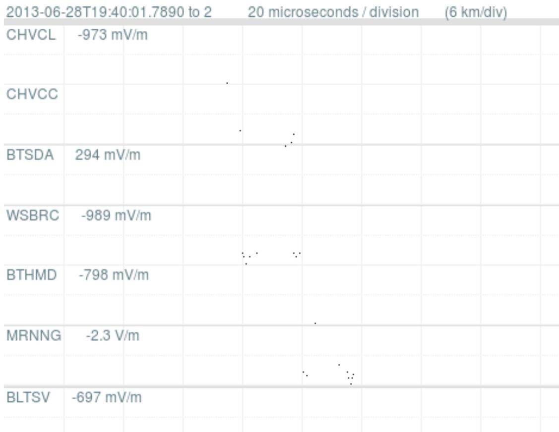
Figure 74: Electric field for twenty fourth (and last) pulse. Negative radiation field, barely visible. Unclear whether this is one or two pulses. The last VHF from this flash was more than 5 milliseconds earlier.
