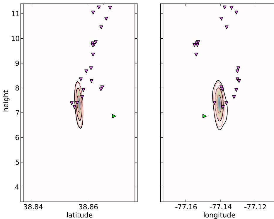
Figure 58: Vertical location of eighteenth pulse. In the latitude versus height plot, it appears that the low frequency pulse is at the lower end of one branch of the channel, and the VHF source is at the lower end of the other branch. Or maybe one or both of these pulses are mislocated.
