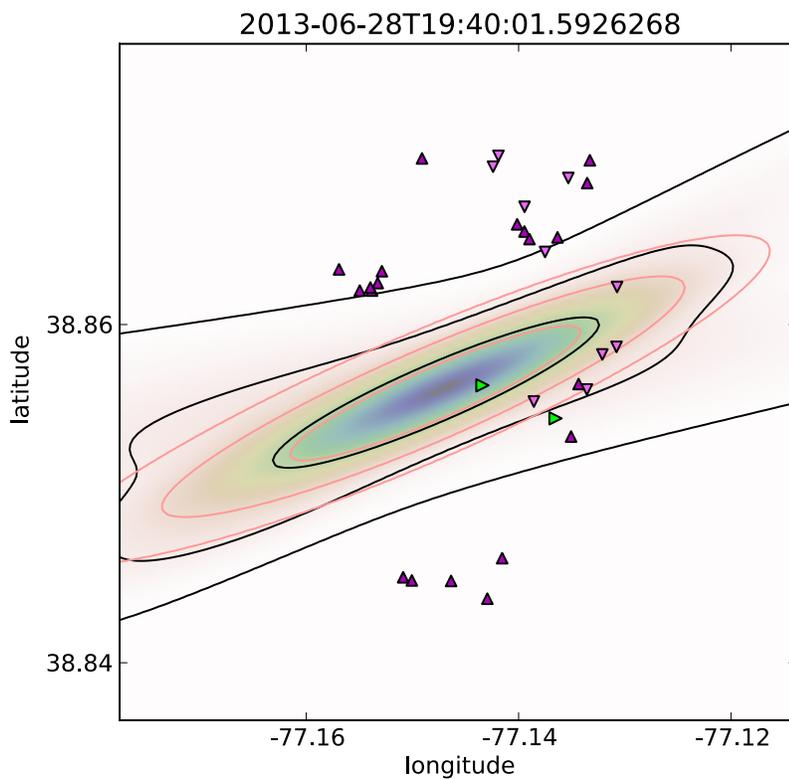
Figure 24: Location of seventh pulse. The location errors are very large; the contours containing 90% and 99% of the total probability density do not fit in the bounds of the plot.
