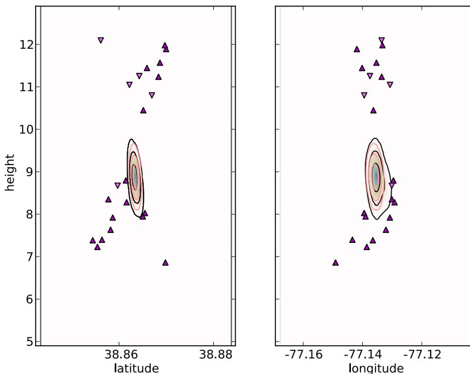
Figure 13: Probability density for vertical source location of the third pulse of this flash. Black constant probability density contours contain 50%, 90%, and 99% of the total probability as before. Red contours show what we would have computed for 50%, 90%, and 99% contours if we had assumed that the timing errors of our system were Gaussian. Triangles show locations of VHF sources identified in this flash. No VHF sources occurred within 5 milliseconds of this pulse.
