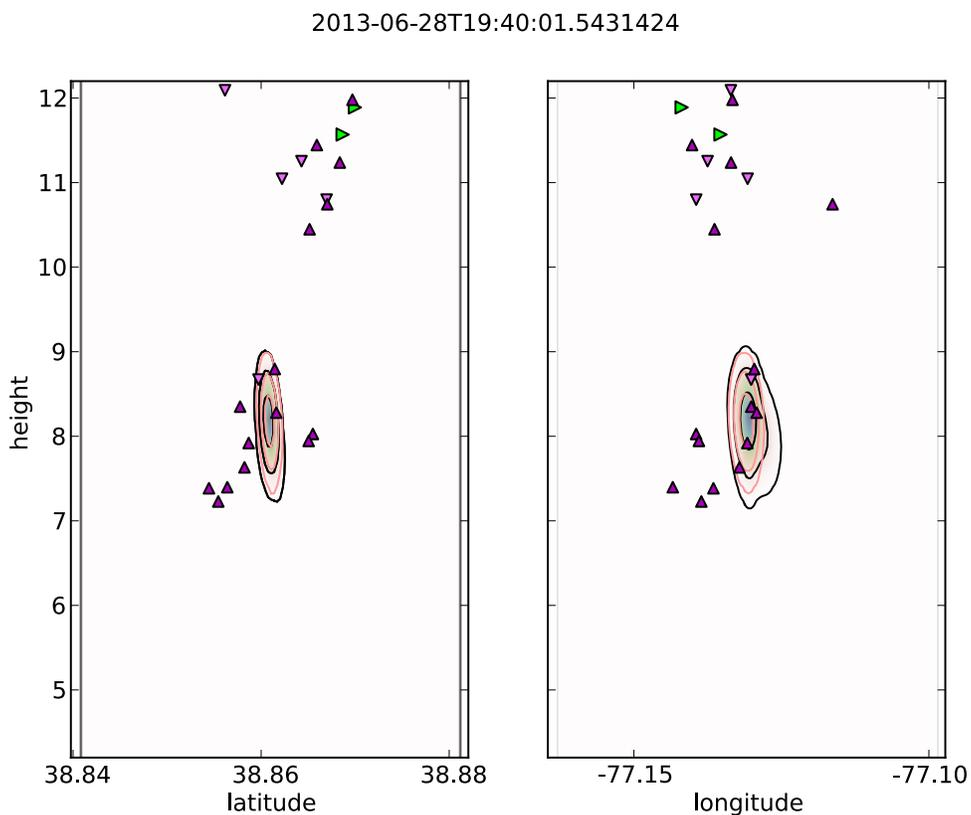
Figure 16: Probability density for height of fourth pulse of this flash. Black and red contours have same meaning as in all the other figures. Triangles show locations of VHF sources identified in this entire flash. Green triangles occurred within 5 milliseconds of this pulse. This is farther east than any previous pulse of this flash. The VHF is in a new portion of the upper end of the channel, the low frequency pulse is in the top of the lower part of the channel.
